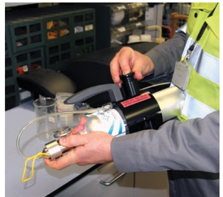
Using the sensor's luminescent spot or tip for dissolved oxygen calibration
